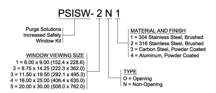
**NOTE:** Window Viewing Size, Type, Material and Finish selections are made by end user to meet final application requirement (MODEL NUMBER SHOWN ABOVE IS AN EXAMPLE).
